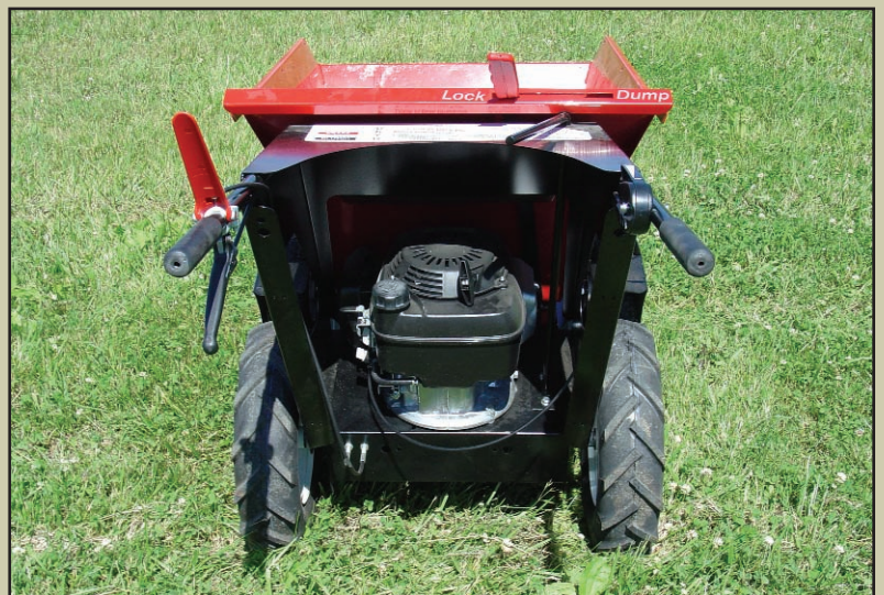
Terra Truck features a Honda engine. The red handle on the left is the safety brake, black handle on the left is the clutch, and the throttle is on the right handle. All are conveniently located and easy to operate.
