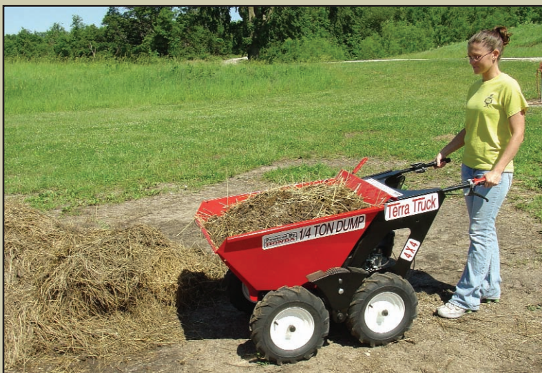
With a manual wheel barrow, the operator has to handle a significant portion of the total weight. With a Terra Truck, almost all of the weight is transferred to the four wheels and none to the driver. You simply steer the machine, not manhandle the weight.
