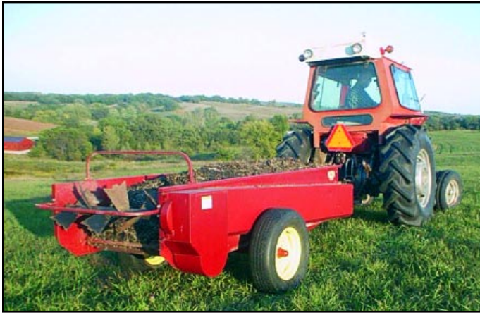
A manure spreader is used to haul manure and waste bedding and then spread the material out over a wide area in a field.
