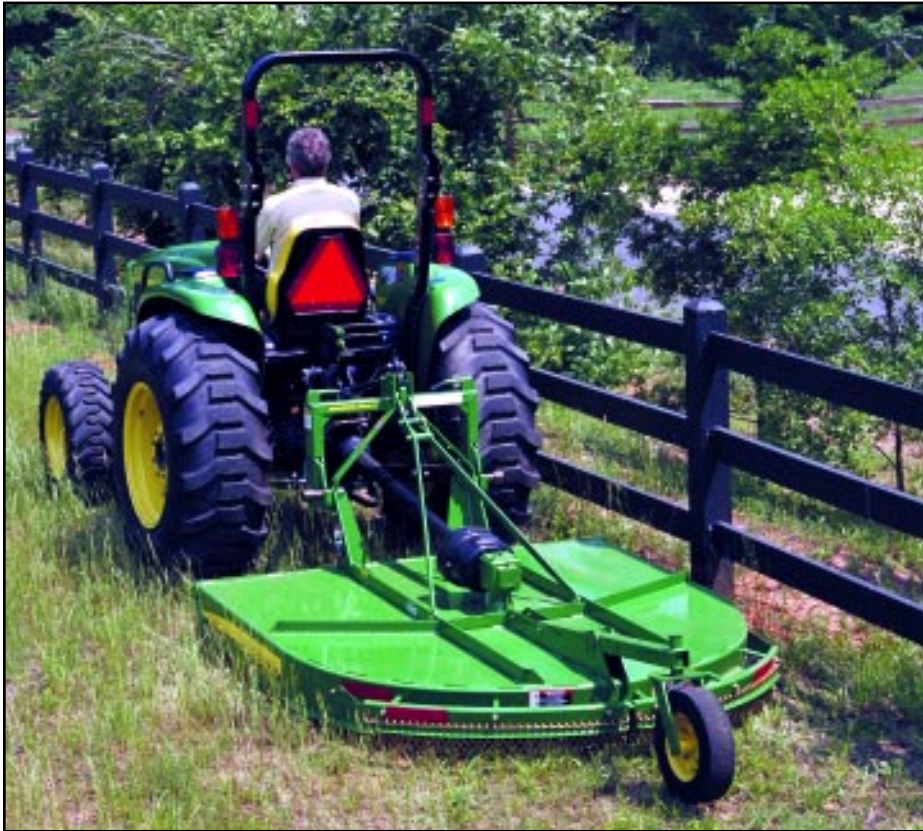
Above, rotary finish mowers are used to cut grass to a lawn like appearance.
