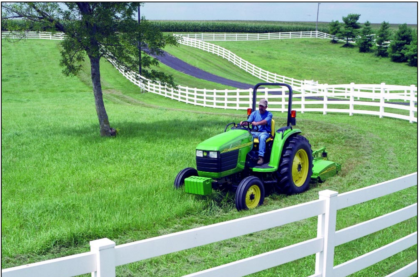
Below, brush cutters are similar to rotary mowers, but they are built much heavier, can cut small trees up to two inches in diameter and are used to mow pastures, weeds, and small brush along fence lines.
