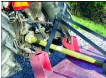
A power takeoff shaft (yellow) is used to transfer power from the tractor to rear-mounted implements.
