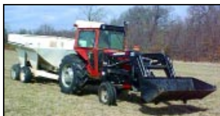
This utility tractor has a front-end loader and is being used to pull a rented fertilizer cart through a hay field.
