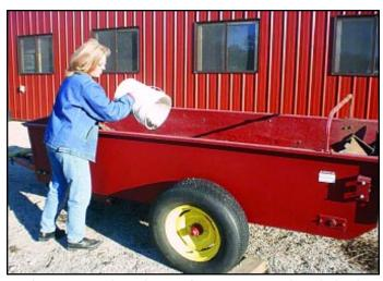
One feature to consider in shopping for a manure spreader is the height of the sides of the spreader. If you lift buckets of manure up and into the spreader, a lower side height is very important.
