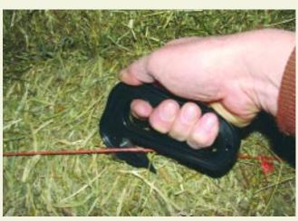
Kaycee Twine Cutter. A specially-designed twine cutter makes cutting the twine off small square hay bales both safe and efficient. The cutter has a handle large enough to even use with gloves. No more fumbling with pocket knives or a cutting knife in the winter. The blade on this cutter is mounted back in the handle to reduce accidents. (\$5)
