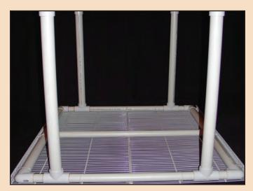
Partially disassemble the table by picking it up and turning it upside down. Then pull the four legs out of the T's.
