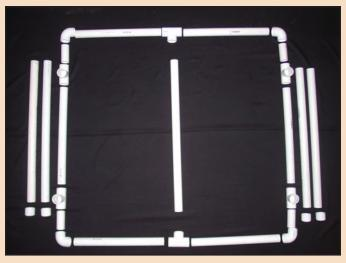
The skirting table frame and legs are made from 1 1/2 inch diameter, Schedule 40 PVC pipe and fittings. Start the project by carefully cutting the pipe to specific lengths and laying out the table top frame for assembly.
