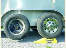
Pull the trailer forward until the good trailer tire is perched on top of the trailer tire changing aid (or back up, depending on which tire you are changing). Set the vehicle emergency brake and turn off the engine.
