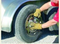
Replace the wheel cover, ensuring that the valve stem opening is properly lined up. Line up the cover so that it almost pops on the wheel. Then, using your gloved fist, firmly tap the portion that is not snapped. It will pop into place. Tap around the cover to ensure that is is firmly in place.
