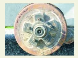
Line up the wheel lugs. A simple trick is to slightly rotate the wheel hub until one of the lugs on the hub is centered at the top. This will make it easier to install the spare tire.
