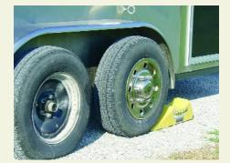
Place the trailer tire changing aid in front of the good front tire on the same side of the trailer as the flat tire. This way, you can pull onto the aid. If the front tire of the trailer is flat, place the trailer changing aid in back of the good back tire and back onto the aid.
