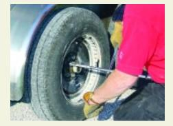
Tighten all lug nuts again with the star lug wrench in the alternating cross type pattern until they are very tight.
