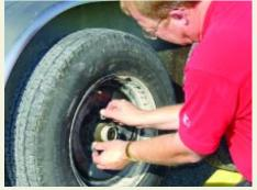
Insure that the tire is pushed all the way back onto the hub. put the lug nuts back on the lugs and tighten to finger tight. Next, tighten the lug nuts with the star lug wrench in an alternating pattern. Start with the top nut, next do the bottom nut, then the nut at the upper left, then lower right, etc. This cross-type pattern will help ensure the wheel is lined up correctly on the hub.
