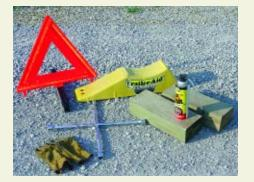
Tire changing tools: leather tools, star lug wrench, trailer tire changing aid, wood tire block, emergency tire sealant, emergency road triangle, and flashlight. Don't forget the spare tire, as well.
