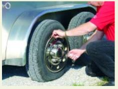
Using a large flat screwdriver, remove the wheel cover from the flat trailer tire.
