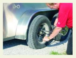
While all trailer tires are still on the ground, use a star lug wrench and loosen all the lug nuts on the flat tire wheel. (Note: if you raise the tire off the ground before loosening the lug nuts with the wrench, they are very difficult to break loose because the wheel will spin freely.) Leave them finger-tight still holding the wheel on the trailer.
