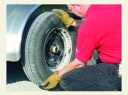
Align the holes in the spare tire to have one centered at the top. Lift the tire onto the hub and wiggle the tire so that it slips onto all the lugs.
